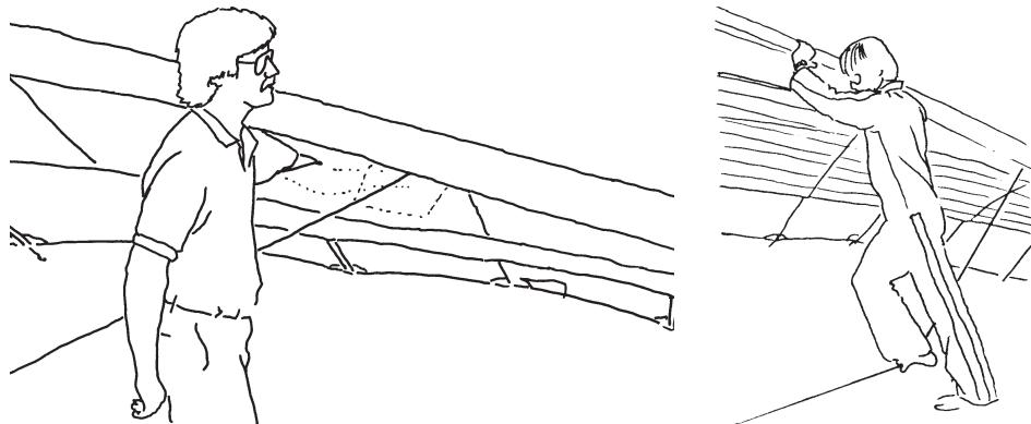
Open the crossbar junction access zipper and look inside, making sure that the safety ring on the junction bolt is in place and that the wires are secure and properly routed. Re-close the zipper.
