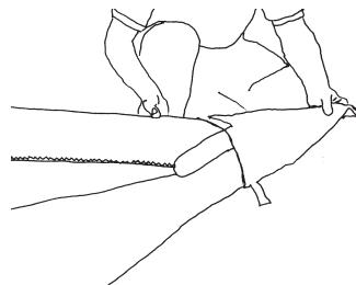
12. Install the plug-on #1 battens by inserting one end through the hole in the bottom surface at the tip and engaging the forked batten tip on the clevis pin standoff on the back side of the leading edge. Secure with a double loop of the 505 batten string.
