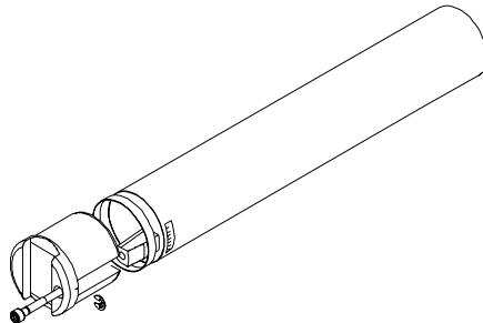
Shims are added to the allen screw type plug by sliding them over the end of the plug before the plug is inserted into the leading edge. The shims are thus visible with the plug installed.
