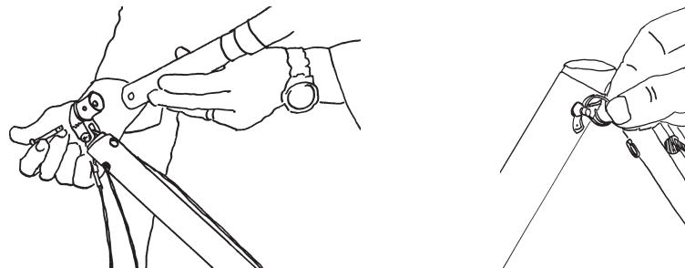
Do not insert the fitting at an angle, and do not force the fitting into the basetube if it does not slide in freely. Check for dirt or damage to the fitting or the inside of the basetube. If the fitting is forced into the basetube, it may be impossible to remove. See your dealer if the fitting becomes difficult to install or remove.
