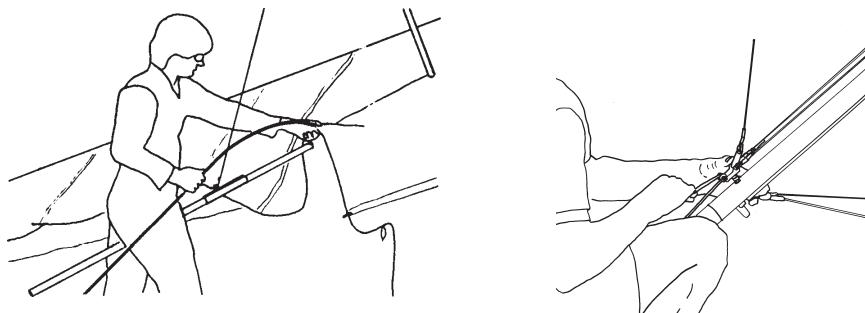
9. Spread the wings all the way and check all cables for any twisted thimbles or tangled cables. Check at this time that no bridle line is caught under the end of an adjacent batten.
