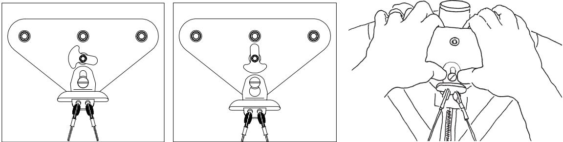
After installing the keyhole tang, rotate the aluminum anchor lock as shown to secure the tang on the bolt.
