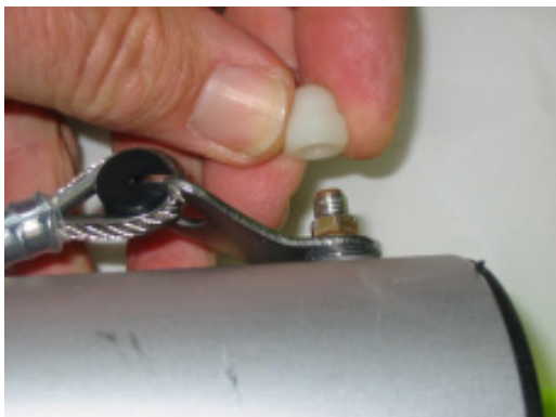
Installation of clinch nut
