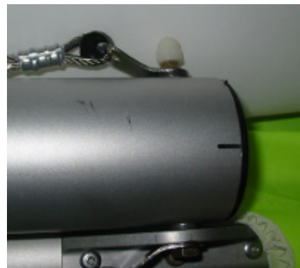
Nylon nut cap installed above clinch nut
