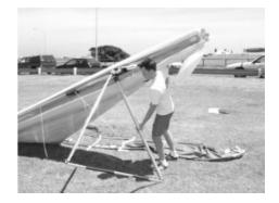
4. Insert the ring of the low er front wires in the Bailey Block making sure that the spring is firmly locked and the wires untwisted.
