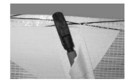
14. Locate the inner and outer wire braced dive struts by placing them inside the sail, below the webbing loop. Note that the action of closing the cord-wise zipper creates the loop necessary to hold the strut in place.
