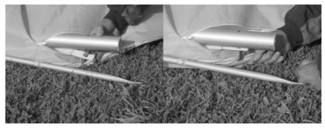
5. Repeat steps 1-4 to install the left hand back section of leading edge. Your Litespeed will now be ready for the standard assembly. Before flight, make a thorough inspection of all tubing and nuts and bolts to ensure no damage has occurred during transportation. (refer to section on pre-flight check).
