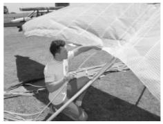
10. Open zipper at sail tip to allow access to inside of sail. Slide fibre glass rod through end of sail and locate in the end of the leading edge. Ensure that the fibre glass rod is pushed hard against its stop.
