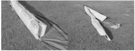
2. Ex pose the leading edge/cross bar junction through the inspection zip. Remove the bubble w rap and tape from the leading edge/cross bar junction and the end of the middle sleeve.
