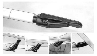
8. Spread the wings all the way and check all cables for any twisted thimbles or tangled cables. At the rear inside of the keel pocket find the sweep (crossbar tensioning) wire. Pull the sweep wire out the rear end of the keel pocket, and check that the sweep wire is not wrapped around the keel. Attach the ring of the sweep wire to the hook, which is placed on the keel tube.
