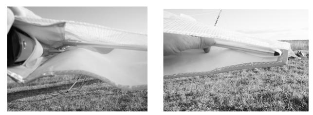
11. The next step is to install the outboard sprogs. To do so swing the sprog away from the leading edge and push it towards the leading edge in to the receptacle. Make sure the sprog sits all the way in the sprog receptacle.
