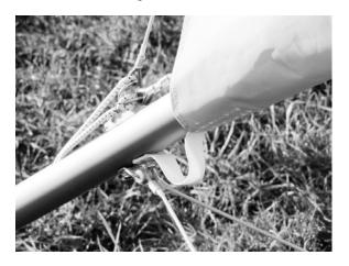
Check the nut of the kingpost channel, which secures the channel to the keel. Check the safety ring and the clevis pin, which secures the kingpost to the channel. Check the safety ring, nut and bolt which secures the hang loop to the kingpost. Check the kingpost top for proper attachment of the bridles and condition of the top rear wire, carabiner and bridle wires.
