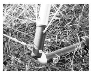
Check the sweep wire for wear where it passes through the kingpost channel.
