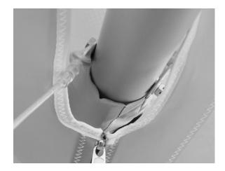
At the left wingtip: Check that the tip lever batten is properly installed.
