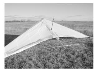
When spreading the wings make sure the washout bridles are not twisted or tangled around the bridle carabiner.
