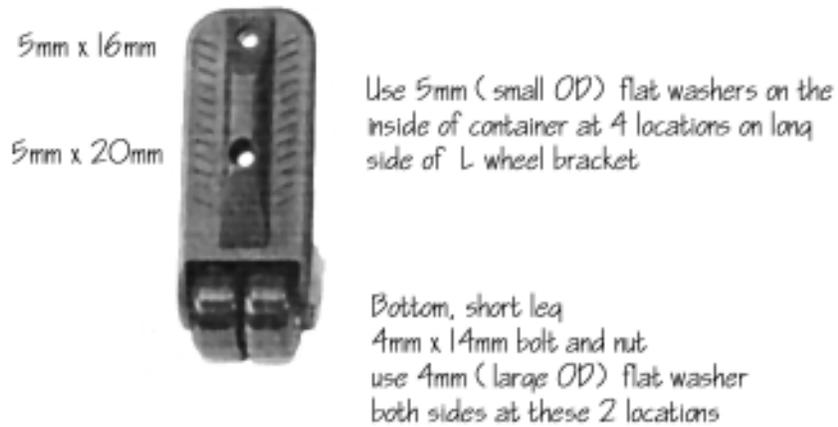
The preferred orientation of the fasteners is with the heads of the screws on the inside of the container and the locking nuts on the outside, however that fastener orientation requires a 5mm metric socket to tighten the nuts. If you don't have a 5mm metric socket, insert the screws from the outside and hold the nuts on the inside with pliers while you tighten the screws.
