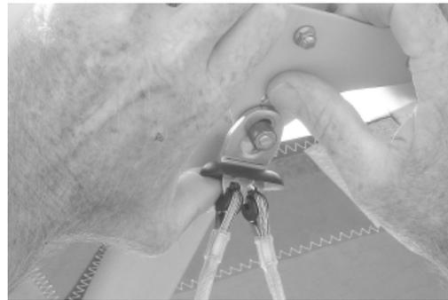
2. Depress the keyhole button lock on the bottom of the noseplate to allow the keyhole tang to be disengaged. Disengage the tang by pulling down on the nose of the glider while pushing up with your thumbs on the plastic tang handle.
