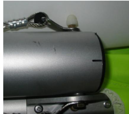
Nylon nut cap installed above clinch nut
