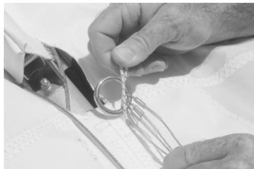
6. Detach the bridle ring from the snap hook, and lay the kingpost down forward against the keel.
