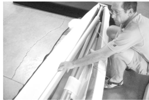
Feed the top side wires into the sail through the holes in the top surface. Swing the outboard crossbars to the rear to align them with the leading edges. Carefully slide the frame out through the nose of the glider. If you encounter resistance, stop and find out what is hanging up.
