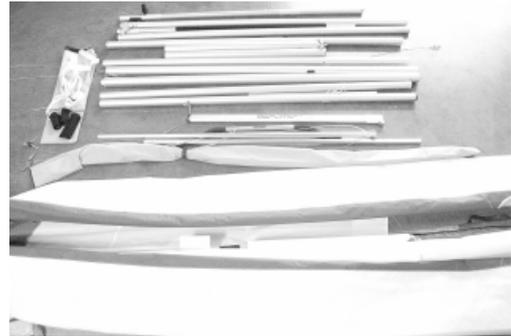
4. Lay the front leading edges / front keel assembly and the inboard crossbars assembly in the box. At each stage of the packing process, use the glider's cover pads, cover bags and any additional materials necessary to pad hardware fittings and protect the tubes from damage or abrasion.
