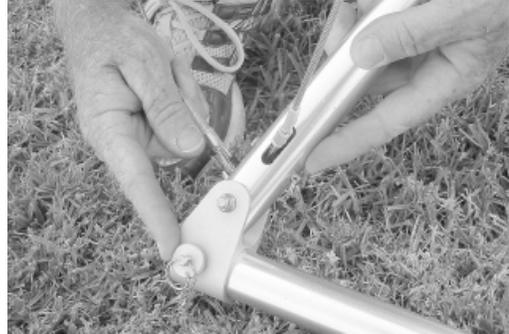
Check the cables at the control bar corners, making sure that all six cables are properly secured and that there are no kinks or twisted thimbles. Check for proper installation of all bolts, nuts, pins and safety rings at the control bar corners.
