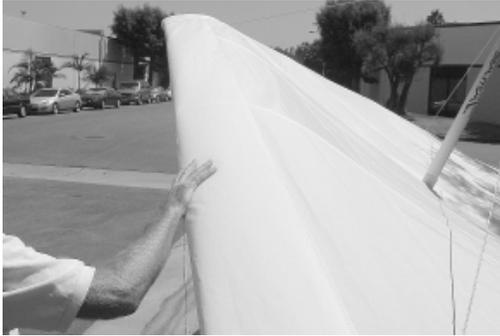
Check the nut which secures the leading edge crossbar bracket to the leading edge, and check the nut and safety ring which secures the crossbar to the bracket. Check that the sail is not caught on the crossbar end, nor on the safety ring, nor on any of the hardware.
