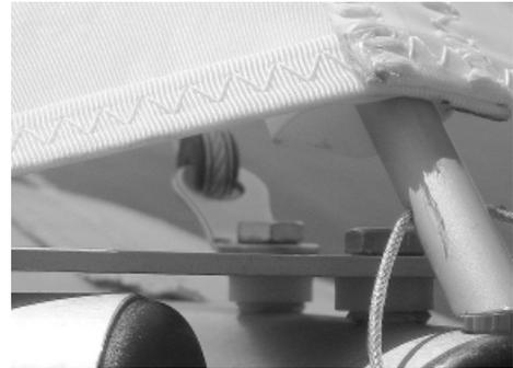
Install the nosecone by pulling the bottom tabs forward and down around the nose, and mating the velcro surfaces on the tabs to those on the sail. Make sure that the nosecone lies as flat as possible, and does not depress the button lock safety feature securing the bottom front wires. (Note - If you hear a flapping sound after launch, it may be that you have forgotten to secure the nosecone. If this happens, don't panic - fly the glider at moderate speed to a safe landing.)
