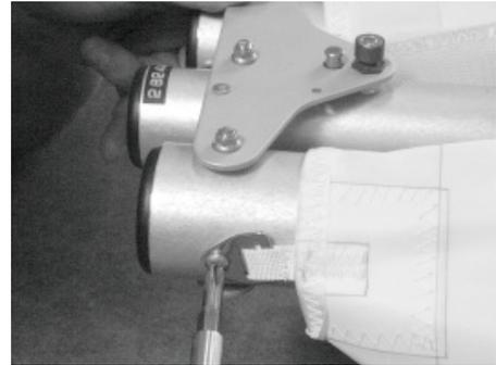
6. Pull straight aft on the rear leading edge tubes to remove the rear leading edges from the frame. (Note - You can skip this step if you are not short-packing the glider).
