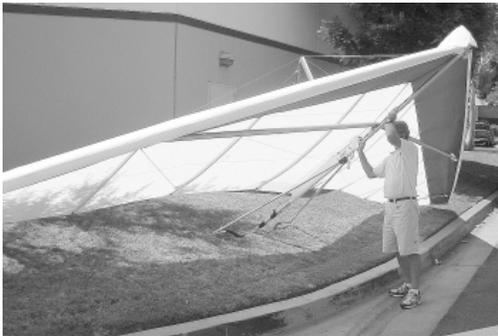
2. Rock the glider forward so that the basket folds rearward and underneath the glider as you gently lower the glider to the ground.
