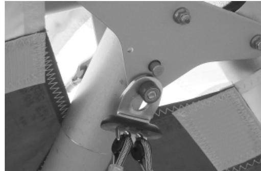
14. Make sure that the spring loaded button lock pops up behind the tang, securing it in place.
