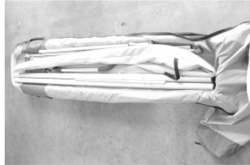
6. Fold another layer of the glider bag over this layer of tubes. Remove the basetube from the control bar. Lay the remaining tubes in the short pack box.
