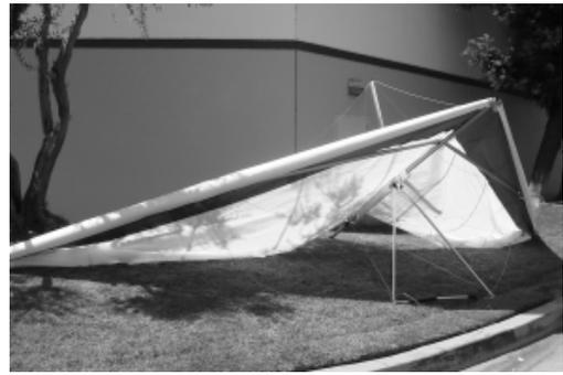
4. Flip the glider upright and set it on the control bar, and remove the glider bag and all Velcro sail ties.
