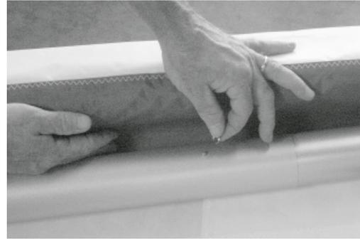
Pull the crossbar center towards the nose of the glider, working it up and down as necessary, to disengage the inboard crossbars from the outboard crossbars. Re-stow the clevis pins and safety rings in the inboard crossbars. When the inboard crossbars are disengaged from the outboard crossbars, turn the inboard crossbar assembly on its side and bring it around one side of the keel tube to remove it from the glider.
