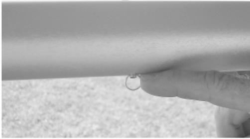
Check that the mid-crossbar clevis pin and safety ring are installed.
