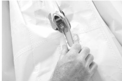
3. Remove the screw from the cap on the top of the kingpost, carefully remove the plastic kingpost cap, and remove the bridle pigtail, top rear wire, top front wire, and both top side wires from the kingpost top. Replace the bridle pigtail and re-install the kingpost top cap and screw.
