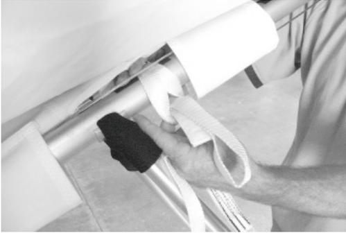
2. Insert a #2 Phillips head screwdriver into the rear bolt securing the control bar apex and kingpost base to the keel. Use a 5/16 box end wrench to loosen and remove the clinch nut that secures the kingpost base bracket to the keel. Replace the nut on the bolt and tighten the nut one half turn so that it does not come loose and get lost. (Note - When removing the nut, use the screwdriver to hold the screw and turn the nut with the wrench, as opposed to trying to turn the screw.)
