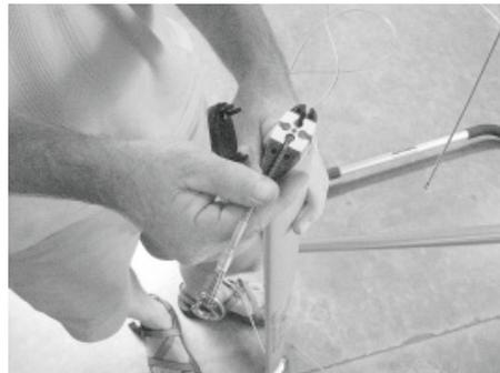
4. Spread out the glider bag, and lay the glider on its side on the bag. Using a 1/2 inch wrench on the keyhole collar and a 7/16 inch wrench on the bolt, remove the bolt securing the bottom rear wire and keel pocket sail mount to the rear of the keel, store the bolt in the tang and re-install the keyhole collar on the bolt, tightening 1/2 turn to secure it against becoming lost.
