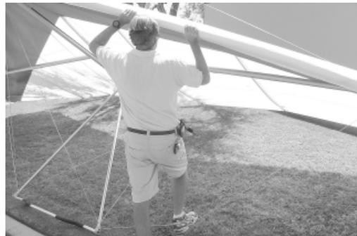
While pushing up on the leading edge between the nose and the crossbar junction, step on the bottom side wire with about 75 lbs. of force. This is a rough field test of the structural security of the side wire loop, the control bar, the kingpost, and the crossbar, and will likely reveal a major structural defect that could cause an in-flight failure in normal operation.
