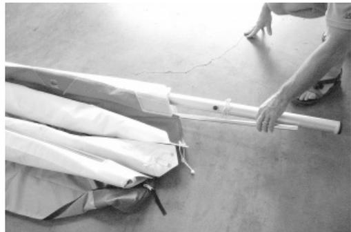
7. Prop the nose of the glider up on the breakdown storage/transport box and spread the wings slightly. Pull the crossbar sweep wire (and attached top rear wire) forward out through the keel pocket. If there are no alignment stickers installed at the joint between the inboard and outboard
