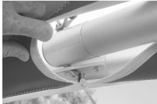
Check that there are no cocked thimbles on either end of either bottom side wire, or on the crossbar end of the top side wire.
