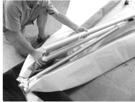
When properly positioned, the crossbar center should lie below the keel (because the glider is upside down) with the central nut on the center hinge bracket joint facing the floor. Install the inner crossbars onto the outer crossbars, matching up the alignment marks, and secure by installing the clevis pins and safety rings. Feed the top rear wires and crossbar sweep wire along the keel through the keel pockets and out the rear of the sail. Install the washout tubes as follows:
