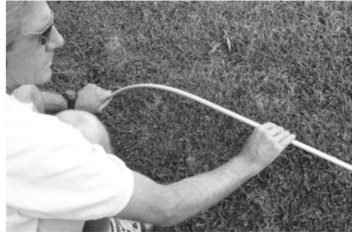
7. Lay out the battens and check each batten for symmetry against the corresponding batten from the other wing. Wills Wing convention is that *black tipped battens go in the right wing and white tipped battens in the left*, except for the straight #1 plug-on battens which may both have the same color tips.
