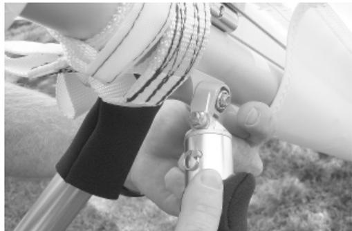
Check the control bar apex bracket hardware, including the clevis pin safeties, the control bar top plug bolts and nuts, and the elbow to apex bracket nut and bolt.
