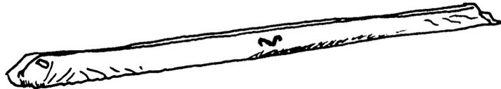
1. With the glider in the bag, lay the glider on the ground, zipper up, with the nose into the wind. If there is more than five mph of wind, or if the wind is gusty, turn the glider slightly more than 90 degrees to the wind direction.
