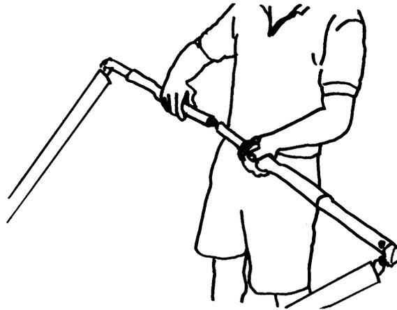
Preflight the folding basetube center hardware at this time, checking that the nuts and coil spring pins are secure, and that the tangs are straight and in good condition.
